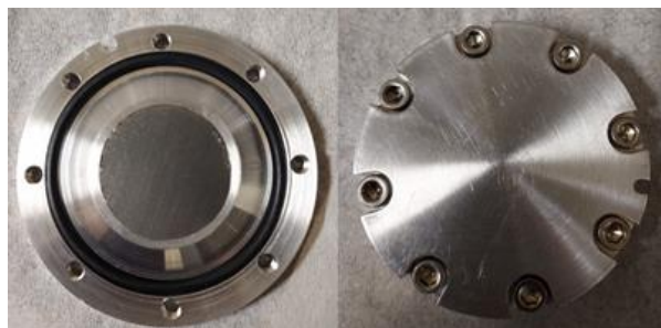
Figure 4.2: Natural lutetium foil enclosed between aluminum target holder and held in place by screws is shown.
